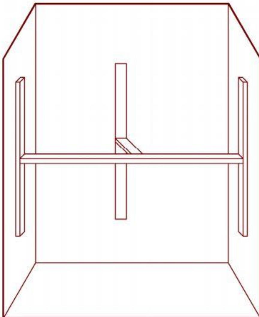
6. Install trim next to the side panels, measuring from the tops of the panels to the floor (if applicable).
