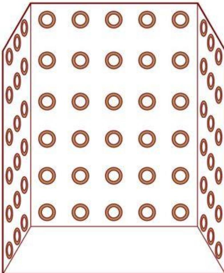
4. Measure the end panels, using the lines you have already made on the walls. It is usually easier to measure the plumbing wall first. You will need to cut the panel to desired dimensions before cutting the plumbing holes. Measure and trim the panel (cut the panel on the side butting up to the back wall-do not cut the outside edge of the panel). Now, measure and cut the holes for the plumbing.
